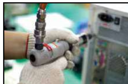
▲ Operation of Auto Shut-Off Screwdriver
