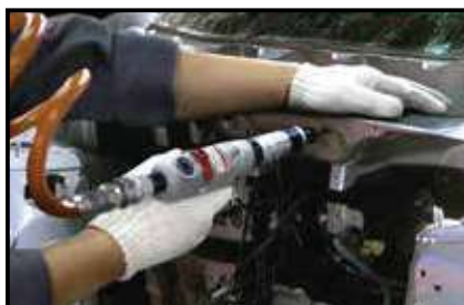
▲ Operation of Auto Shut-Off Screwdriver
