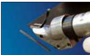
▲ Operation of Air Metal Shear
