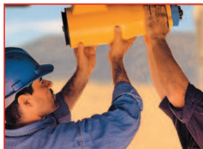
An ST650BP03R31 starter is shown being mounted on a CAT3512 used on a mine haul truck.
