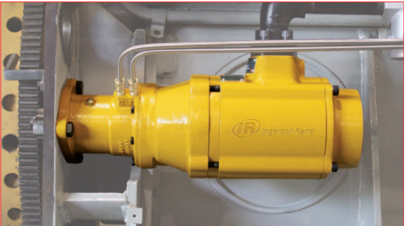
An ST1060CP03R25S on an EMD 16-645 genset application.
